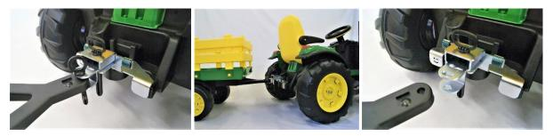
The adapter consists of a main support (1), a bottom reinforcement plate (2) and a back-adapter (3). It is delivered with one  $\emptyset$ 10 and one  $\emptyset$ 14 mm plastic pin. Fastened by one M10 nut without modifications on the tractor.
